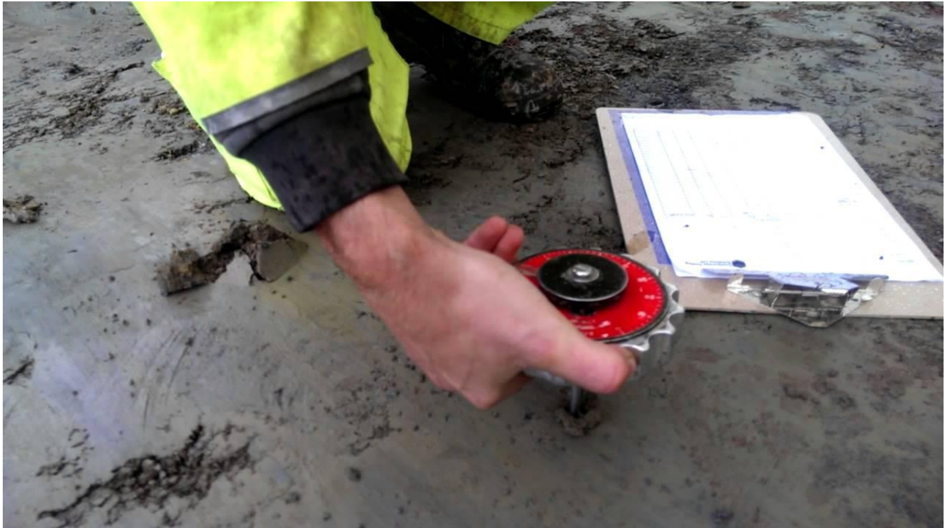
Photo showing the method of testing soil strength with a shear vane
